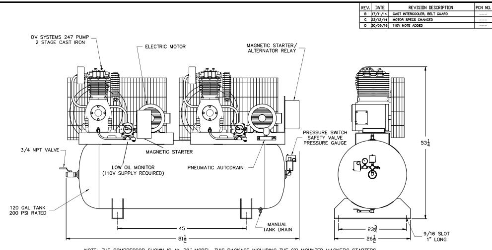
NOTE: THE COMPRESSOR SHOWN IS AN 'XL' MODEL, THIS PACKAGE INCLUDING THE (2) MOUNTED MAGNETIC STARTERS, ALTERNATOR RELAY, (2) OIL MONITORS, AND (1) PNEUMATIC AUTODRAIN.
