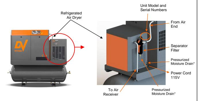
\*Drains will discharge automatically under pressure. It is recommended that pneumatic drain tubes be anchored and filtered as per your local municipality regulations.
