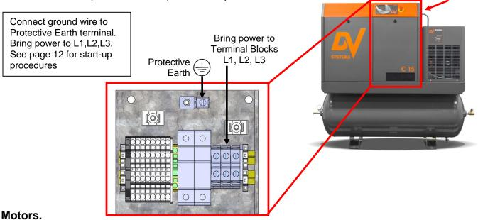
Wiring must be done in a manner that the full Motor nameplate voltage +/- 5% is available at the Motor terminals during start-up. Contact your local Distributor or Service Centre if additional information is needed.
