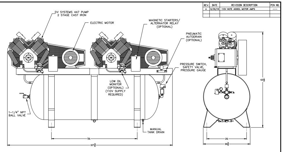
NOTE: THE COMPRESSOR SHOWN IS AN 'XL' MODEL, THIS PACKAGE INCLUDING THE (2) MOUNTED MAGNETIC STARTERS, ALTERNATOR RELAY, (2) OIL MONITORS, AND (1) PNEUMATIC AUTODRAIN.
