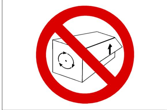
Never operate the unit with open doors or loose access panels.
