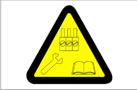
Check and, if required, re-tighten connection terminals. For further details, see the operating instructions.
