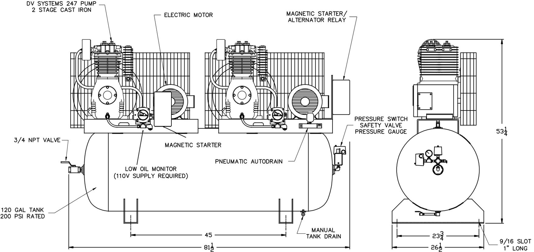
NOTE: THE COMPRESSOR SHOWN IS AN 'XL' MODEL, THIS PACKAGE INCLUDING THE (2) MOUNTED MAGNETIC STARTERS, ALTERNATOR RELAY, (2) OIL MONITORS, AND (1) PNEUMATIC AUTODRAIN.
